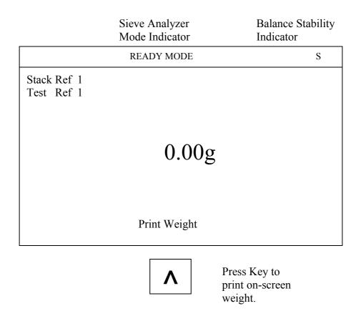
\*\*\*Make sure the Balance Stability Indicator is stable. It will flash to indicate that the instrument is on an unstable platform or in a draft.
