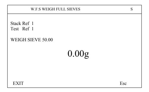
Place the sieve on the weigh pan, then wait until you hear two beeps and the screen asks you to remove the sieve.
