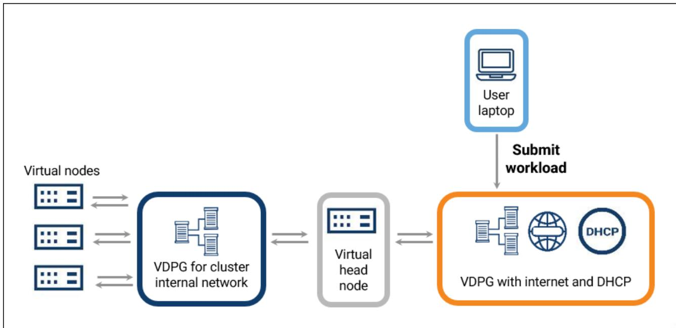
Figure 2: End users log in and use the cluster in the same as they would access any other HPC cluster
