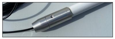
**Step 4.** Attach the base coupling to the Extender base using the three provided screws and a flathead screwdriver (not provided). Note: If desired, before installing the base coupling to the Extender base, dab a small bead of the provided lubricant to the screws to prevent galvanic corrosion.
