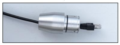
**Step 3.** Connect the Ethernet base mount coupling to the base of the Halo Pro Extender and line the screw holes up
