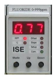
Each module has a 3 digit display and LEDs to indicate operating modes. The module is programmed by the use of 3 keys located on the front panel.
