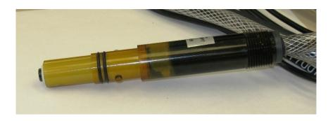
The combination fluoride sensor includes both the measuring and reference electrodes with electrolyte, electronics and a high-impedance PVC organic membrane system in a sealed plastic body. As such there are no replaceable or serviceable items in the sensor. The only service required is occasional cleaning and calibration.
