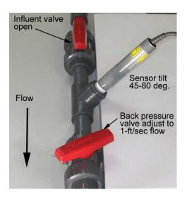
The sensor orientation should be between 45 and 80 degrees above horizontal to prevent air bubbles becoming trapped near the ion selective membrane or on the sensor tip. Sensors should NEVER be mounted with the sensor tip pointing straight down, horizontally, or pointing up as this may cause a bubble on the sensor tip and lead to erratic or unreliable readings.
