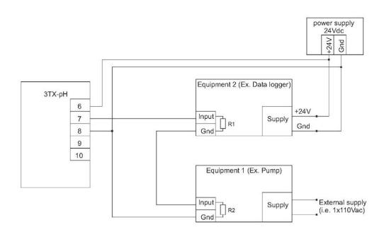
Note: R1 and R2 are internal resistors. R1 + R2 <  $500\Omega$
