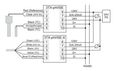
The lead providing +24VDC power always goes to terminal 6 and the 4-20mA current loop output is always sent from terminal 7. The DC common (ground) is shared as terminal 8. The current loop output is sent from terminal 7 and return to terminal 8 (ground / DC common). The FX-300 transmitters are always energized on terminal 6 with the DC ground of the 24VDC power supply (a.k.a. rail) always being the (shared) terminal 8.
