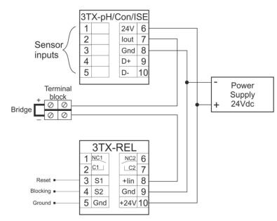
3.5 Alternate wiring schematic for adding multiple devices to the 4-20mA transmitter output loop.
