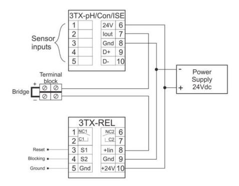
If you wish to "insert" an external device into the current loop, it can be done by removing the bridge jumper and connecting the two terminals to the external device ("+" to device input and "-" to device output, which may also be device ground). If no external device is to be connected, the bridge jumper must be in place to ensure normal operation of the FX-300-REL relay module.
