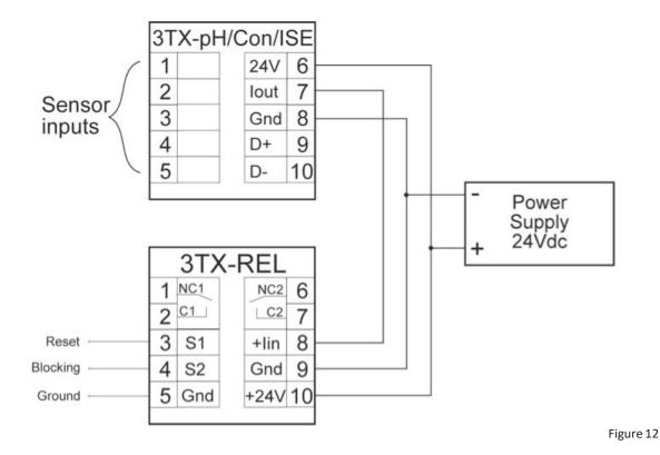
**Note**: An alternate wiring configuration is required if the 0/4-20mA transmitter output is to be first (also) sent to another data acquisition or control device.
