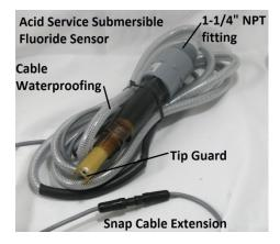
The sensor should be mounted at a 15-45 degree angle to prevent an internal air pocket from contacting the sensor tip resulting in erratic and unreliable readings.
