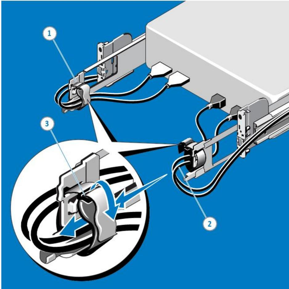
**Figure 58. Routing the Cables**
