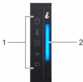
*Figure 14. Left control panel without optional iDRAC Quick Sync 2.0 indicator*
