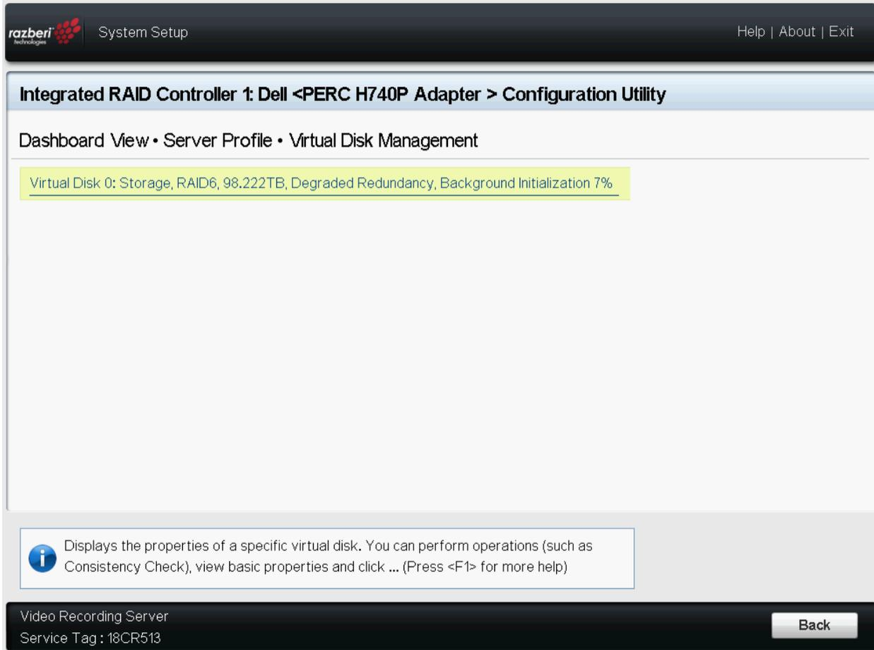
**Figure 64. PERC Adapter: Virtual Disk Management**
