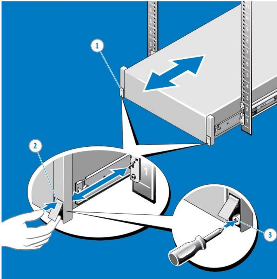
**Figure 57. Engaging and Releasing the Slam Latch**
