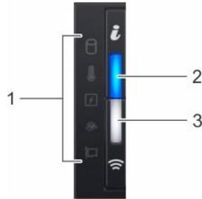
**Figure 25. Left control panel with optional iDRAC Quick Sync 2.0 indicator**
