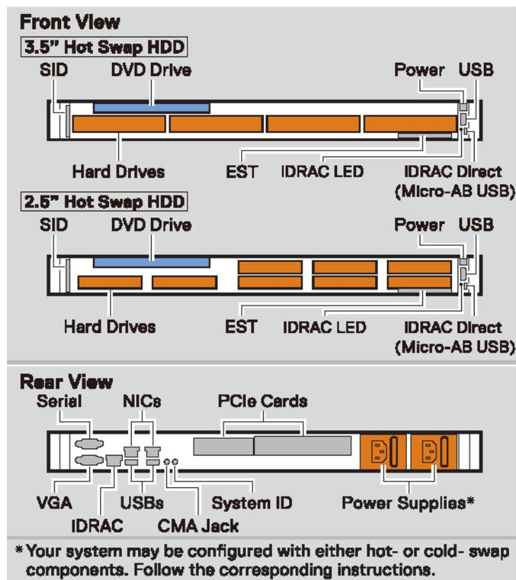
**Figure 48. Front and Rear Touchpoints for M4**
