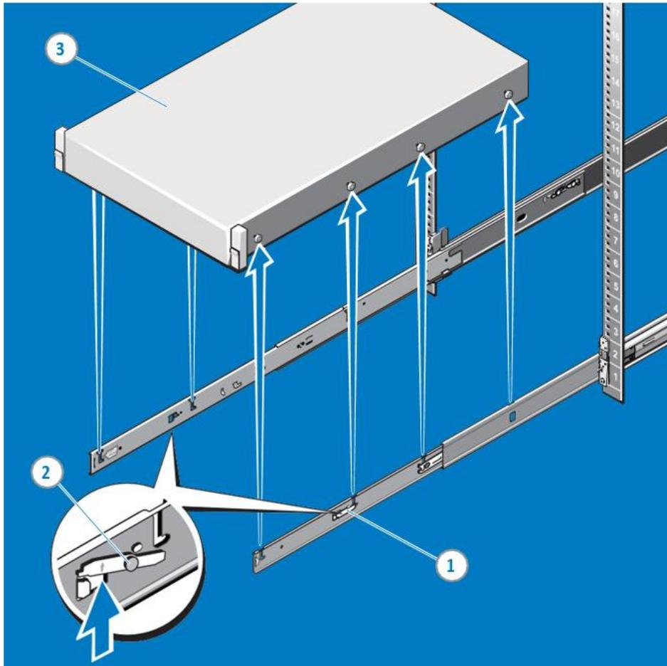
**Figure 56. Removing System from the Rack**
