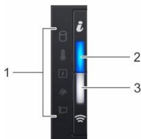
*Figure 15. Left control panel with optional iDRAC Quick Sync 2.0 indicator*
