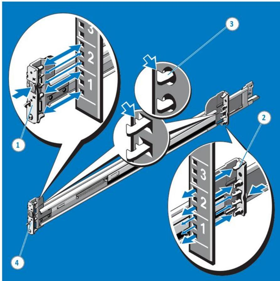
**Figure 53. Installing and Removing Tool-Less Rails**
