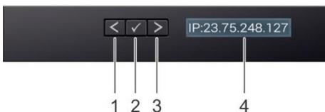
Figure 9. LCD Panel Diagram
