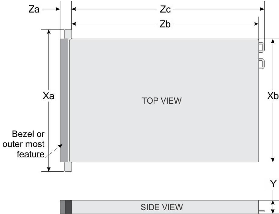
Figure 49. System Dimensions for V8, V12, and V14
