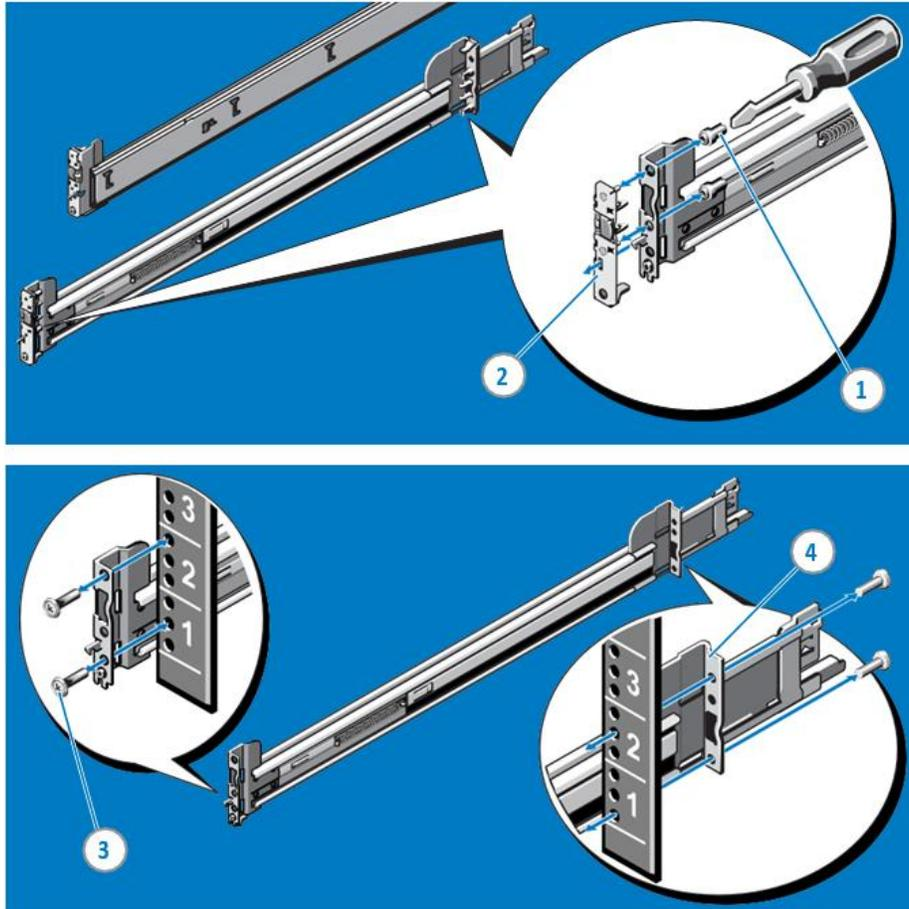
**Figure 54. Installing and Removing Tooled Rails**
