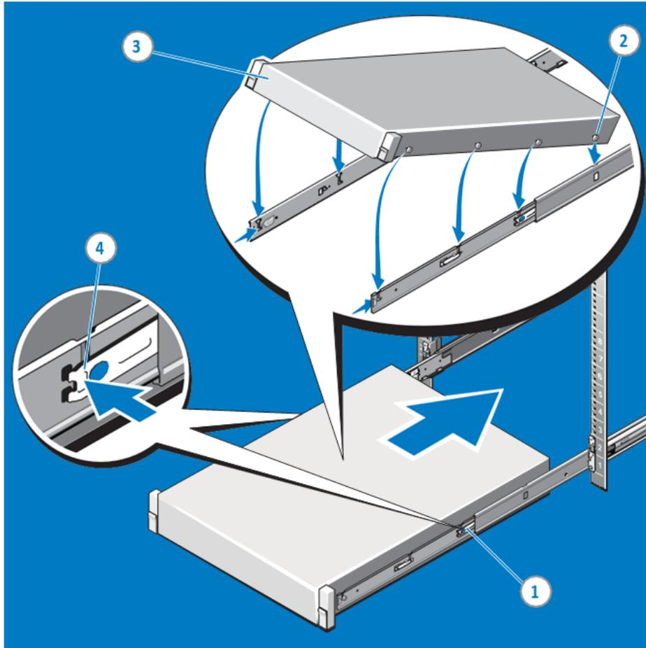
**Figure 55. Installing the System in a Rack**
