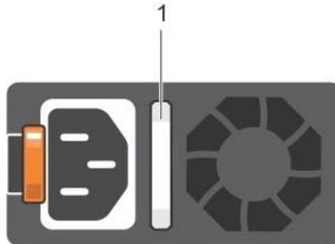
**Figure 8. PSU Indicator Diagram**
