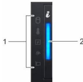
*Figure 24. Left control panel without optional iDRAC Quick Sync 2.0 indicator*
