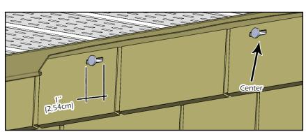
If you need to attach the siding in an area other than the installation hole, create a 1"(2,54 cm) long slot to allow nailling. Always nail in the middle of the slot.
