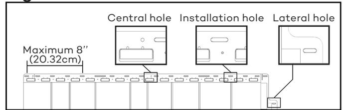
2-Never hammer or screw the fasteners in completely; leave a gap of 1/16"(0.16cm) between the nailing channel and the fastener's head (Figure 2). Always use non-corrosive nails or screws with a head of 0.4"(1cm) in diameter and a body of 0.150"(0.38cm) in diameter and penetrate through the solid surface by at least 1 1/4"(3.18cm) and into a solid substrate by at least 7/16"(1.11cm).
