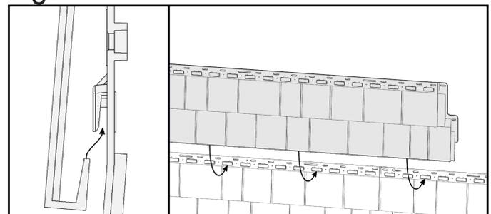
4-When using a finish trim (J-channel, Outside Corner Post, etc.), leave a space of 1/4"(0.64cm) between the trim and the TandoShake (Figure 4). The required opening for finish trim is 3/4"(1.91cm).
