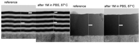
TEM micrographs of Picosun's ALD nanolaminate and oxide encapsulants after one month soaking tests in 87 °C PBS. No corrosion observed (image source ULIMPIA-project).
