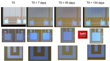
Microimplant electronics protected by Picosun's ALD HfO<sub>2</sub>. No changes after soaking in 87 °C PBS for over 3 months, which correlates to over 10 years in human body (image source CEALeti, France, InForMed project).
