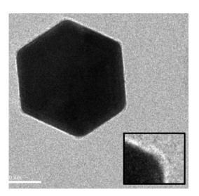
ALD offers lots of alternatives for particle surface modification and functionalization. Left: ZrO<sub>2</sub> beads ready to be coated in a PICOSUN® ALD reactor. Right: Cu nanoparticles with uniform, conformal ALD oxide coating. Coating thickness on Cu nanoparticles 1 nm.
