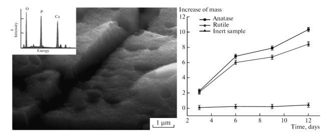
Left: SEM picture and EPMA analyses of Ti plates with anatase TiO<sub>2</sub> coating, after soaking in SBF for 6 days Right: Comparison of HA formation on plain and ALD TiO<sub>2</sub> coated Ti samples in SBF<sup>(\*\*)</sup>.
