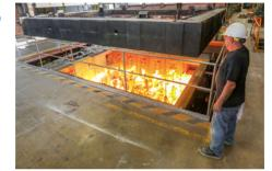
In this furnace we can test the fire endurance of a wide range of assemblies.
