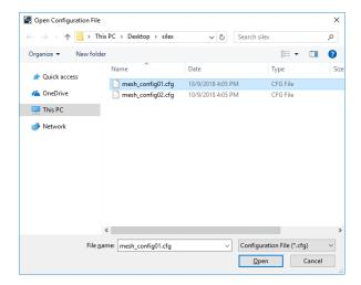
**7.** The selected configuration file is displayed under **Configuration File Name**. Repeat **5-6** to specify the configuration file for all BR-400AN units.
