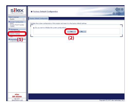
**3.** When the factory default configuration is completed, BR-400AN is automatically restarted. When the restart is completed, the POWER LED turns green and the WLAN LED turns or blinks orange/green. BR-400AN will run in a normal mode then.
