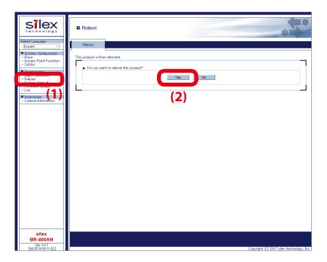
**3.** The restart is completed when all LEDs turn off and then the POWER LED turns green and the WLAN LED turns or blinks orange/green. BR-400AN will run in a normal mode then.
