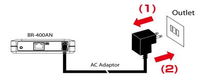
**2.** When the POWER LED turns green and WLAN LED turns or blinks orange/green, the restart is completed. After the restart, the BR-400AN will start in a normal mode.
