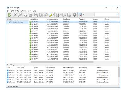
As shown in the image below, AMC Manager® can configure IP address and write the same setting to several units at once.
