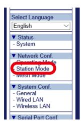
**6.** Configure each setting according to the Access Point to connect (1) and click **Submit** (2).
