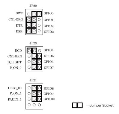
If the left side of jumper pin is shortened with a jumper socket, the special function is enabled. If the right side is shortened, the pin can be used for ordinary GPIO. In the example above, GPIO 0 is the ordinary GPIO, whereas GPIO 1-4 are set to special functions.
