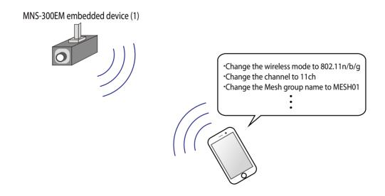
Also, AMC Manager Mobile can copy the Mesh network setting of other Mesh devices to use it to correct the configuration of the isolated device.
