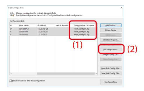
**9.** Specify the IP address range to configure for MNS-300EM units (1). When the setting is finished, click **OK** (2).
