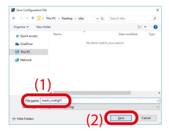
After the configuration is saved, the screen of the step 4 is displayed again. To create a configuration file for each Mesh network group, repeat the step 4-6.
