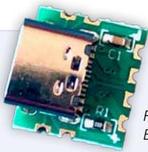
Figure 1: USB-C Adapter Board included in the kit.
