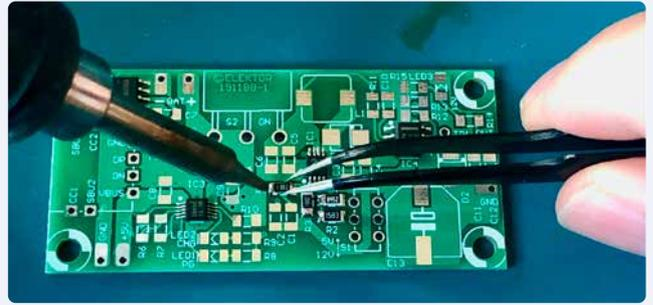
Figure 2: Soldering the resistors to the board.
