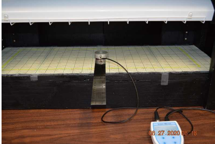
Figure 15. Test Set-Up for Irradiance Mapping
