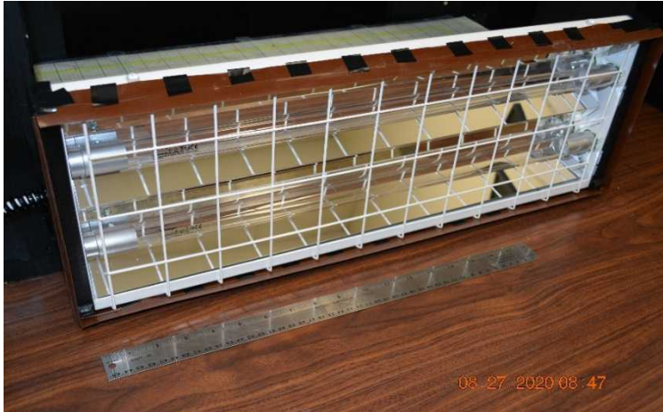
Figure 12. Underside of Lamp with Attached Flexible Sweep
