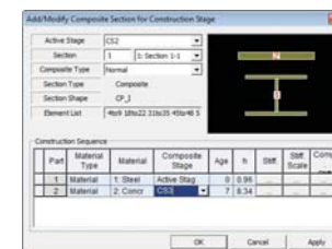
Composite section for construction stage to simulate composite action with 1-D element
