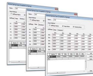
6x6 mass, stiffness and damping matrices to simulate dynamic soil-structure interaction
