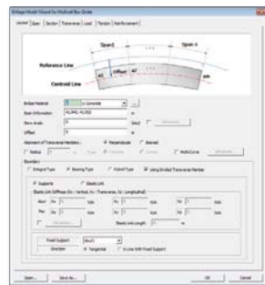
Defining bridge layout with span information and bearings data
