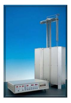
The DL 4000 Dilatometer is an automated instrument for determining the swelling proprieties of hard coal when heated under standard conditions: dilatation and contraction are obtained by inserting a pencil of powdered coal, formed under pressure, in a narrow tube topped by a piston and reading the displacement of the piston as a function of the temperature.
