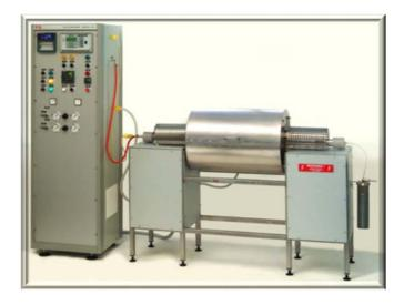
**LTD Test system** is designed and manufactured for the testing of Low Temperature Disintegration of Iron Ore according to the following international Standards:
