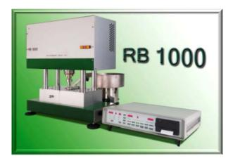
The RB 1000 Iron Ore Pellet Crushing Strength Determinator is an automated system for the determination of the crushing strength of fired iron ore pellets and reduced iron ore pellets, according to ISO 4700 Standard and ASTM E 382-83 Standard.
