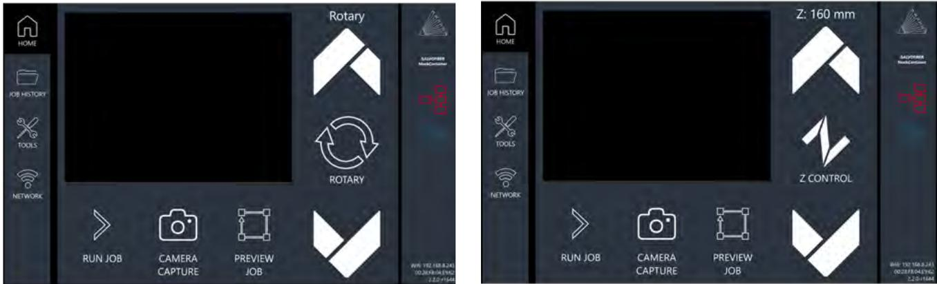
Make sure when using the friction-type rotary that the object placed on it is level for a proper engraving. In rotary mode, engravings can only be made through rastering. In RE3 the rastering speed is what determines how quickly the rotary turns. The distance that the rotary will engrave is dependent on the height of the image that is being engraved. To engrave the entire circumference of the object then the height of the image should be equal to the circumference of the cylindrical object.
