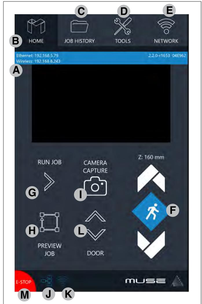
RetinaEngrave v3.0 has a rotary mode you can switch to. The rotary should be connected to the Muse Pandora before it is powered on. Once you engage rotary mode in RE3. The “Directional Jog” button will change to a “Z-Axis” symbol. Tapping on the “Z-Axis” symbol will change to the “Rotary” symbol. The arrows will now control the rotary.
