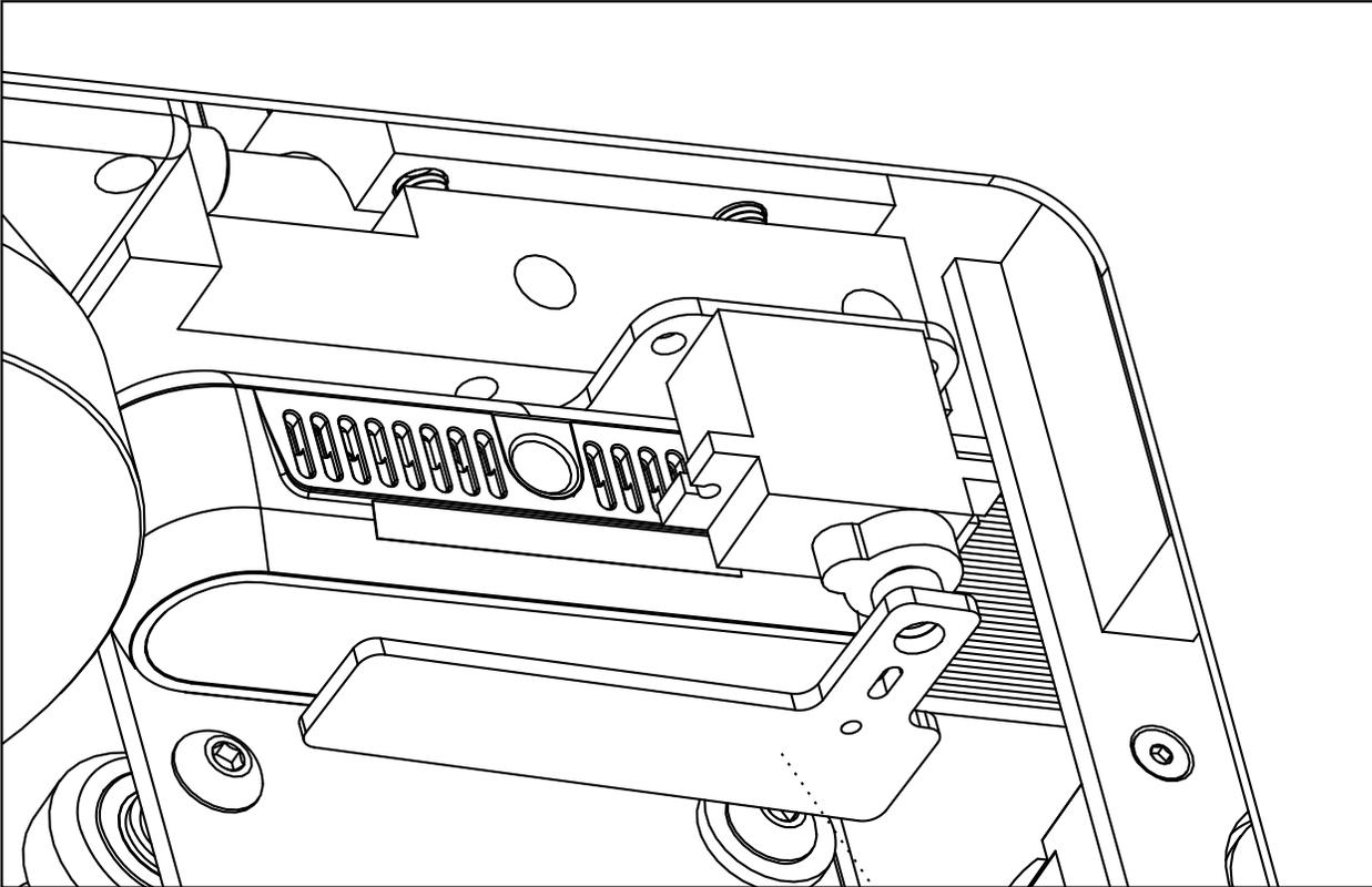
Depicted is the covered position, The camera will be in this position anytime the laser is being used. It will return to the open position after the job finishes.
