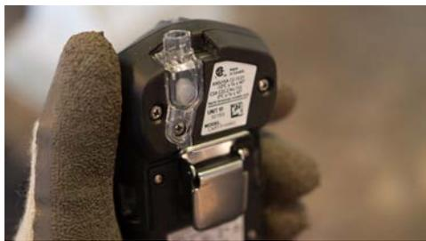
Blackline's in-house hardware and firmware teams completed the majority of work required to complete and submit the final G7 pump cartridge for intrinsic safety certification. This new cartridge expands beyond previous diffusion-based cartridges, enabling users to remotely sample an atmosphere of a tank, sewer or other confined space in order to understand whether potential gas hazards are present. The internal pump draws air samples from the remote location through up to 100 feet of tubing.
