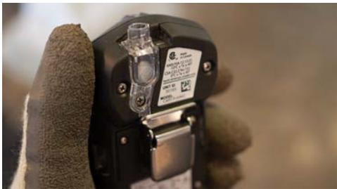
Blackline's in-house hardware and firmware teams completed the development work required and submitted the final G7 pump cartridge for intrinsic safety certification. This new cartridge expands beyond previous diffusion-based cartridges, enabling users to remotely sample the atmosphere of a tank, sewer or other confined space in order to understand whether potential gas hazards are present. The internal pump draws air samples from the remote location through up to 100 feet of tubing.
