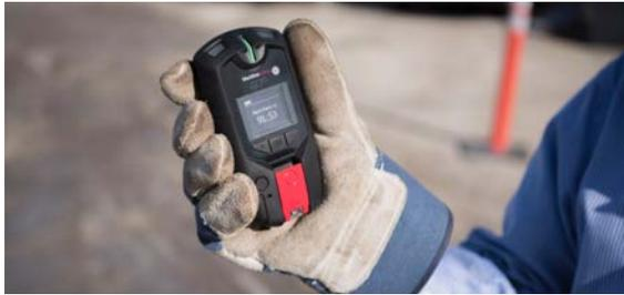
Blackline’s G7 product line supports lone worker monitoring applications with or without the requirement for gas detection. For dedicated lone worker monitoring, G7 devices are fitted with a Standard Cartridge rather than a gas sensor cartridge. Safety monitoring options offered by G7 devices for lone worker includes True Fall Detection®, no-motion (man-down) detection, missed employee check-in, SOS latch and a silent SOS button.
