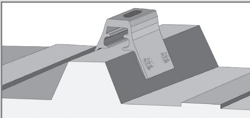
All pre-punched holes must be used to achieve tested strength. Due to varied applications, mounting hardware is not furnished with part.
