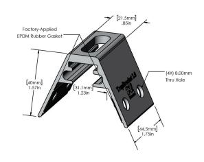
Designed to fit Kingspan KS1000RW and similar roof profiles
