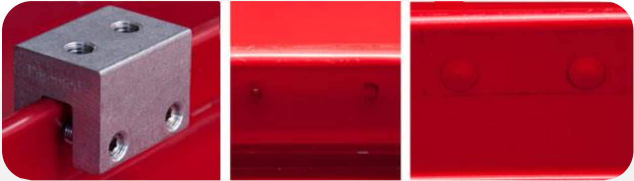
S-5-S; typical “snap seam” profile (this one by AEP); 24-gauge Galvalume; Kynar 500 paint; screw tension: 140 inch-pounds. The darkened areas are a combination of shadow and metal oxide deposits on the surface of the paint.
