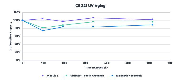
ASTM 4459: Q-Sun XE-1, 0.8 W/m² at 420 nm, 55 °C ASTM D638: Type V, 1 mm/min, average values represented
