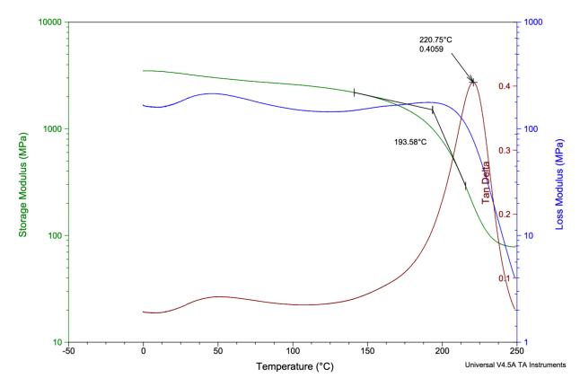
Standard: ASTM D4065 Instrument: TA DMA Q800 DMA Mode: Tension
