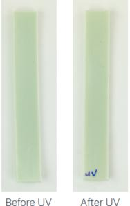
ISO 4892-1/4892-2: Xenon-arc lamp, 1.2 mW/m<sup>2</sup> at 420 nm, 70 °C, 6 hours
