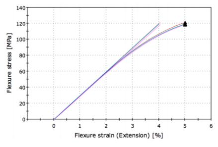
Flexural test method: ASTM D790-B, 40mm span, sample thickness: 3.18mm, dry
