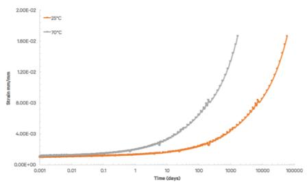
Creep TTS test method: TA Q800 DMA, single cantilever mode, 30x15x3.2 mm sample, 0-125°C sweep at 5°C increments with 5 minute isothermal and 10 minute deformation, 2 MPa applied load, dry
