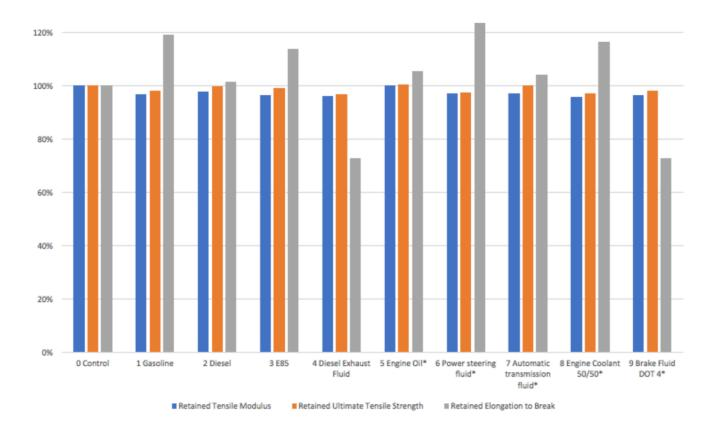
**Treatment Method:** Samples submerged in test liquid for 30 minutes at 23 °C or 50 °C (starred) then removed from test liquid and allowed to sit at ambient room temperature conditions for 1 week (samples were not wiped). **Test Method:** ISO 527-2, Type I, 5 mm/min
