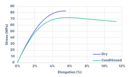
Conditioning method: Conditioned 2 weeks, 23°C/50%RH. ASTM D638 Type V dogbones
