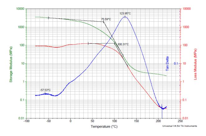
Standard: ASTM D4065 Instrument: TA DMA Q800 DMA Mode: Tension Sample Dimensions: L=20mm, W=10mm, t=1mm (rectangular block) Strain Amplitude: 0.1% (linear regime of viscoelasticity) Oscillation frequency: 1 Hz Temperature Range: -100°C to 200°C
