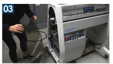
On the opposite side of the control panel, remove the clear side panel so you have access to the screws in behind.
