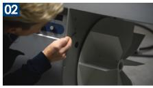
To the right of the control panel you'll see 4 screws. Remove the 1st and 3rd ones.
