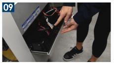
The harness in the middle connects back to the fan, blade and tumbler VFDs and the harness on the right connects back to the linear actuators for the machine tilt.
