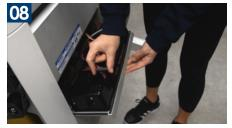
The back of the control panel has three wiring harnesses plugged into it. The harness on the left is the group of wires connected to the sensors. Note, this harness has a bypass attached to it which may be used for diagnosing and troubleshooting issues.
