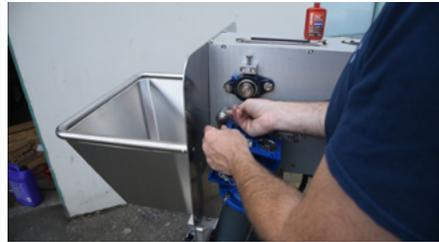
Look down the hole of the gearbox to make sure everything is lined up, then slide the whole assembly on, but leave room to install the rest of the hardware. With a bit of loctite on the bolt, pass it through the bracket and the spacer, then roll the motor until the bolt lines up with the hole in the side plate and start tightening the bolt by hand to ensure it doesn't get cross-threaded, then tighten the rest of the way with the socket.
