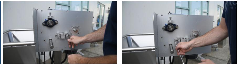
Loosen off the two adjustment bolts so there is a gap between the bolt and the blade block.
