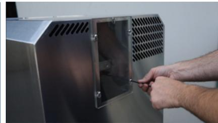
Replace the cover over the chipper and tighten each of the screws.
