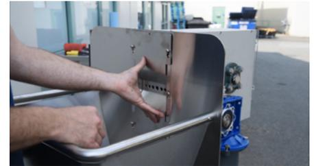
Next we'll reinstall the 4-bolt flange bearing. Make sure the grease fitting is at the top. You may need to grab the chipper from behind and lift it to get the flange bearing to fit into its recess, then line up the 4 holes, add loctite to the first few threads and replace the 4 bolts, tightening each once they've all been installed.
