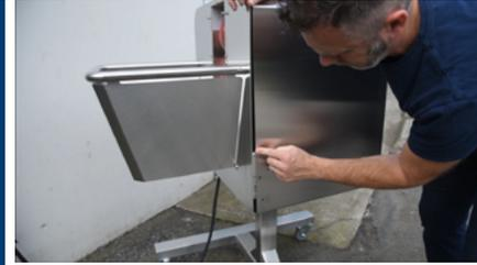
To release the cover, pull down on the shrouding at the bottom, then pull off and release. Repeat on the opposite side, then slide the cover off the MBX.
