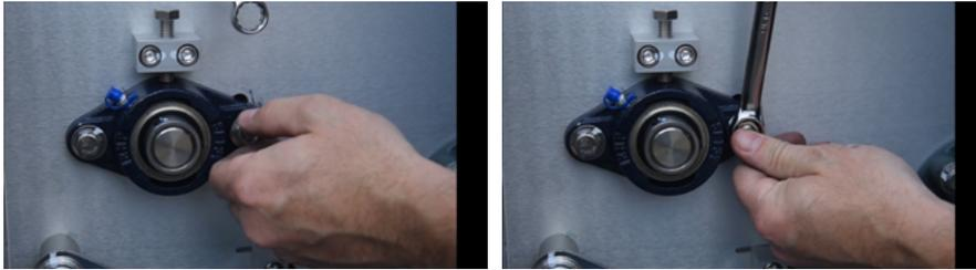
Tighten the bolts on each side of the bearing on both sides of the machine, then snug down the top bolt which will prevent the bearing block from vibrating and coming loose.
