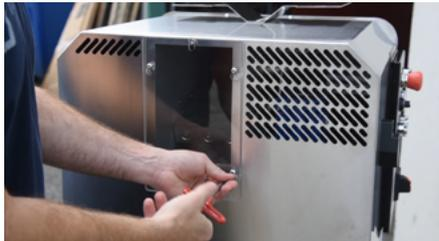
Using the same 5/32 allen wrench, remove the cover over the chipper and set aside.
