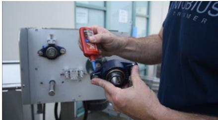
Make sure that the plastic bushings are installed in the 2 bolt lower flange bearing. Add loctite to the two bolts, then slide the bearing onto the shaft.
