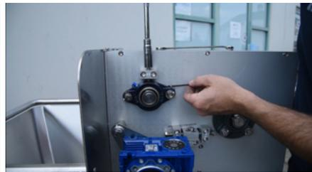
Start tightening the adjuster bolts on the top of each of the upper roll bearing blocks with the 9/16 socket. As you tighten the bolts, it will start to expose a slot where the bolt goes through. You want to tighten the bolt until you can fit a 1/8 hex key in the opening. That's when you know the rolls are adjusted correctly. Repeat the same process on the opposite side.
