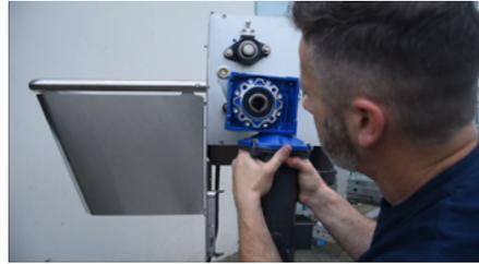
Turn the shaft of the lower flange so that it aligns with the key way on the motor gearbox. With the gearbox on about 1/2 an inch of the shaft, take the key and hold it in the key way
