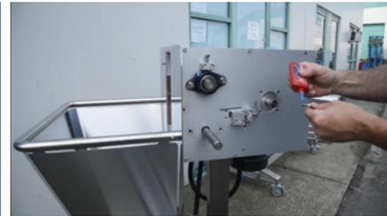
Using blue loctite, replace all seven of the screws on the side plate. Get them all started, but don't tighten until all seven are in place. You can then go back over each and snug them all down, then go back a third time to tighten them.
