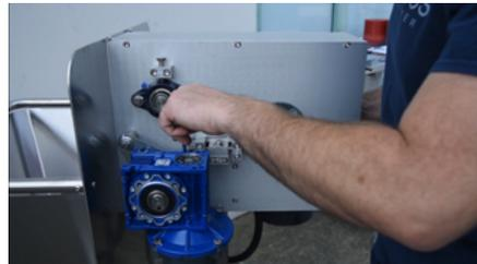
Once both are installed, with safety glasses on, put the circlips back on making sure they're seated in the groove all the way around, then slide the spacer washers back on.
