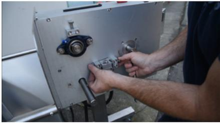
Then tighten the bolts on either side – as tight as you can with your fingers. Once all of the bolts are secured, we'll come back to finish the chipper blade assembly.
