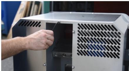
Remove the centre screw with the 3/16 allen wrench, and the 2 button-head screws at the bottom of both side panels.
