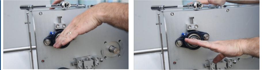
Once loose, the tension is off the rollers and the flange will float up. They pivot down to tighten and pivot up when they're loose.
