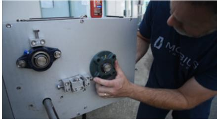
Next we'll reinstall the 4-bolt flange bearing. Make sure the grease fitting is at the top. You may need to grab the chipper from behind and lift it to get the flange bearing to fit into its recess, then line up the 4 holes, add loctite to the first few threads and replace the 4 bolts, tightening each once they've all been installed.
