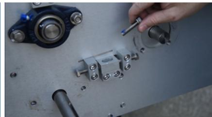
Tighten one of the bolts by hand, then pivot the other side up slightly to get that bolt started, then slide the bearing tight against the plate. Continue to thread the bolts by hand, then tighten with the socket.
