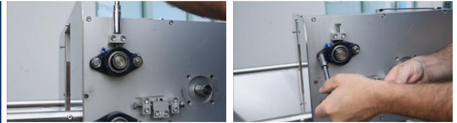
Release the tension off the rolls by loosening the top bolts on the upper 2-bolt flange bearings on both sides of the machine, then loosen the flange bolts on either side
