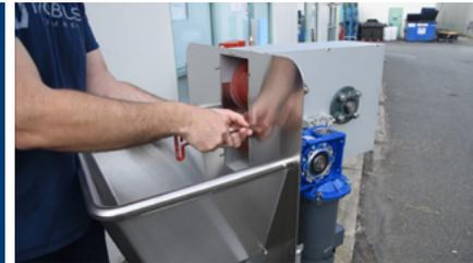
To remove the side plate, use the 5/32 to unscrew the 3 screws on the right side of the rollers.
