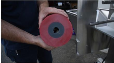
The bottom roller has a keyway. Line that up with the key and slide the roller on.
