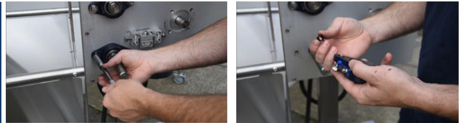
Next remove the lower flange bearing. There are 2 little plastic bushings inside the bearing – be careful not to lose those as you pull the flange off. Set the bearing off to the side.
