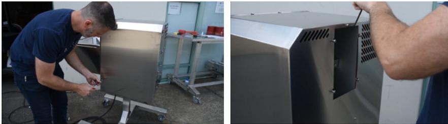
Install the 2 button head screws on the bottom of each side, but don't tighten yet, then thread the centre screw at the top of the chipper side.
