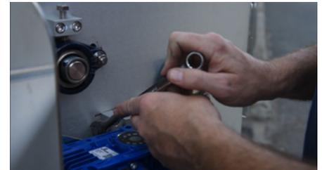
Make sure that the plastic bushings are installed in the 2 bolt lower flange bearing. Add loctite to the two bolts, then slide the bearing onto the shaft.
