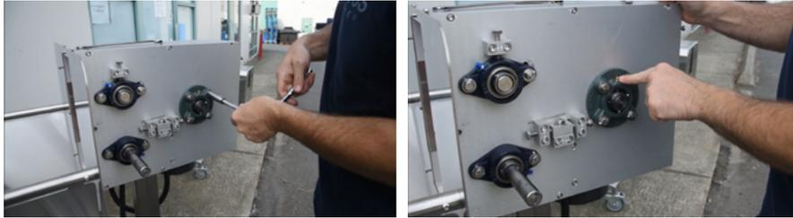
Remove the 4-bolt flange bearing for the chipper using the 9/16 socket on each of the 4 bolts. Note that the grease fitting is at the top – this is where you'll want it when you put the flange back on.
