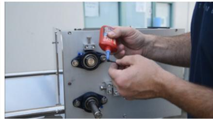
With all the flange bearings installed, you want to remove each of the 6 set screws (2 in each bearing), add a bit of blue loctite, then reinstall them using the 1/8 hex wrench. The 4-bolt flange bearing uses the 3/32 hex wrench.
