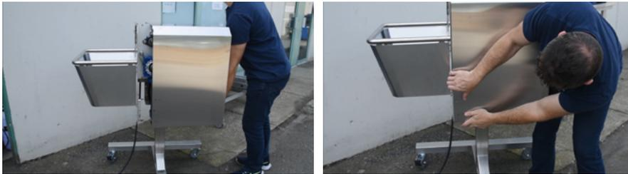
Put the shrouding back on. Make sure that the hooks on the bottom of each side go into the holes.
