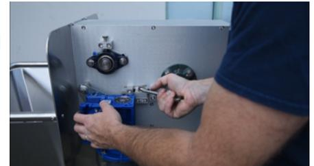
Using blue loctite, replace all seven of the screws on the side plate. Get them all started, but don't tighten until all seven are in place. You can then go back over each and snug them all down, then go back a third time to tighten them.
