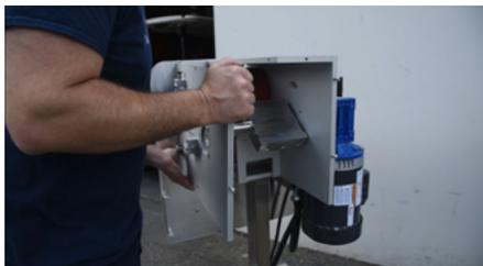
Replace the side plate making sure that all of the holes and two shafts line up properly. The top bearing will need to be moved up to line up with the shaft. Once aligned, the plate can be pushed on the rest of the way.
