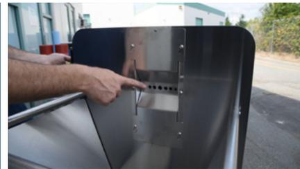
Turn the machine on and allow the rollers to rotate in the forward direction while looking through the holes in the dieplate. Then switch directions
