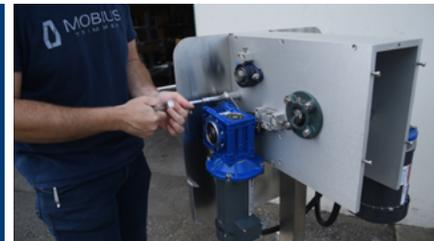
Next, remove the motor with the gearbox using the 9/16 socket. Be careful not to lose any of the parts – there's an aluminum spacer, and a bolt with 2 washers.
