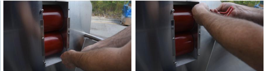
Replace the plate on the side of the rollers with the short screw. The 2 longer screws hold the dieplate in place – they can just be threaded loosely for now, but the middle screw can be tightened up.
