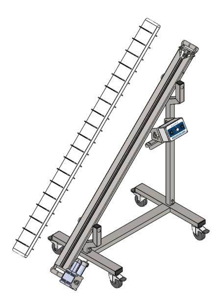
7. Install a SIDE PANEL on each side of the conveyor by aligning the circular cutouts with the THROUGH STOPS and THROUGH BARS. Simply slide each panel down onto the pucks to install it on the conveyor.
