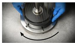
Slide the tumbler end cap at the bottom into the matching profile at the base of the spreader. Rotate clockwise to lock in place.
