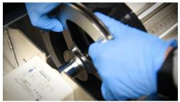
Lift the left end cap and slide it towards the motor to align the drive cone. Rotate the assembly to align the drive pin with one of the holes in the spreader plate. As you do so, the shaft at the knob side should fall down into place on the plastic support.
