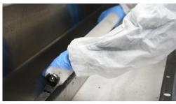
Install the soiled M108S brush into washer by clicking each end of the brush into the receiving clips on the lid. These work the same way that they do in the M108S lid.
