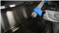
Remove the brush by grasping it at both ends and pulling gently to release it from the clips. Rinse off and set aside to dry. We recommend using the end bearings as support during drying so that the bristles do not dry flat.
