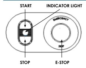
**E-STOP** - Prevents accidental start-up, used for servicing and removing components.
