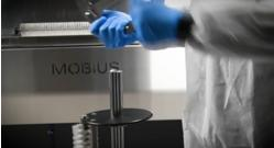
Remove the locking disk from the main shaft of the spreader.
