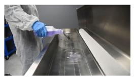
Begin by filling washer basin approximately half full with warm or hot water. The fill slots on the motor mount plate will prevent you from over-filling the basin. It is recommended that water temperature not exceed 65°C (150°F).
