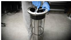
Holding the tumbler end cap on the bottom end to keep locked into place, rotate the knob on the locking disk clockwise to tension the tumbler. The wires must be taut for cleaning.
