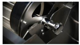
Lift the spreader at each end and lower it into the basin, resting the knob-end on the plastic support on the right-hand side.
