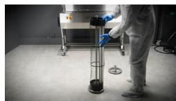
Slide the tumbler over the main shaft of the spreader and replace the locking disk on the shaft. Don't tighten yet!
