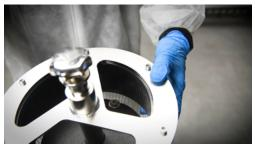
Lift opposite tumbler end cap up and interlock with matching features on the locking disk.
