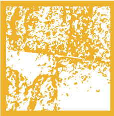
SPLIT FACE Natural grain split, produced by hydraulics or wedges and shims.
