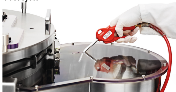
"Clear product without stopping" spheronizer air blast system
