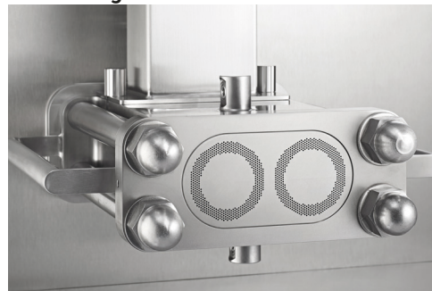
Axial configuration with 1 mm die holes
