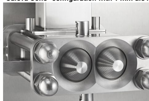
"Caleva Cone" configuration with 1 mm die holes
