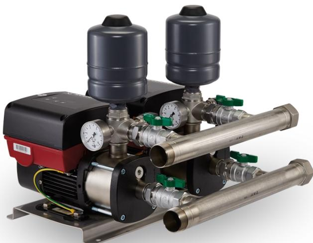
**The Grundfos CMBE Twin is a booster pump for water supply and commercial boosting applications. The CMBE Twin Booster system consist of two CMBE pumps connected in parallel and mounted on a base plate with a Grundfos built manifold. The CMBE pumps will alternate to ensure the same number of operating hours until high flow is needed, and the pumps will run together.**
