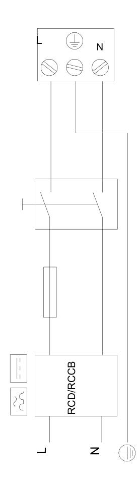
with mains switch, backup fuse and additional protection
