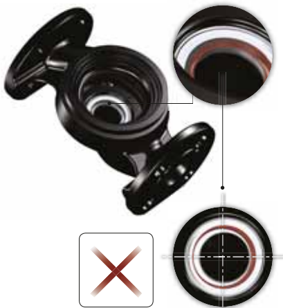
Fig. 10 Incorrectly centered sealing system
