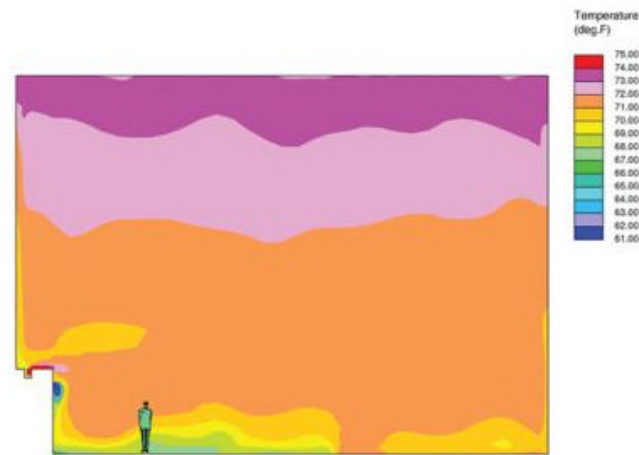
Figure 2: A computational fluid dynamics comfort analysis allows for a detailed look at comfort conditions throughout the space.
