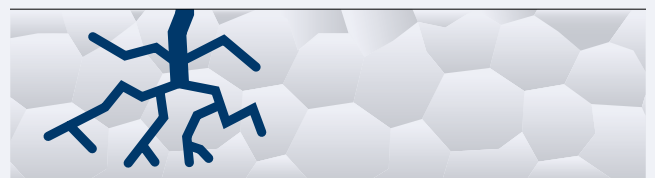
Fig. 1.6.10: Stress corrosion cracking
