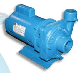
**Series GN Base-Mounted Centrifugals Pumps** are available in 1750 RPM, with capacities to 1100 GPM, heads to 95 feet; and in 3500 RPM with capacities to 950 GPM, heads to 380 feet. The base-mounted pump models are rated for use on inlet pressures to 100 psi, and case working pressures to 200 psi, with suction sizes from 1½" to 5", and discharge sizes from 1¼" to 4".
