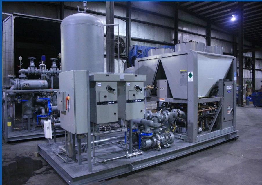
*EnviroSmart System Controllers use adaptive logic to continuously monitor system and weather parameters and make real-time fine adjustments to VFD speeds, system set points, and equipment sequence points to assure the lowest kW per ton of output.*
