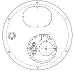
The above drawings of pit and basin cover plates for Type VSP Sump Pumps show standard arrangements of Simplex and Duplex Units for both circular and square plates. Square plates are usually furnished for concrete pits, while circular plates are normally furnished for cylindrical cast iron and steel basins.
