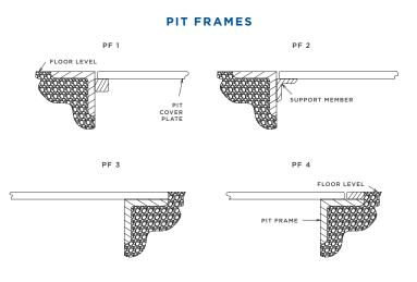
**Type PF-1:** furnished as standard for square and rectangular pits. Permits frame and cover to be installed flush with finished floor. Has bar support for cover.
