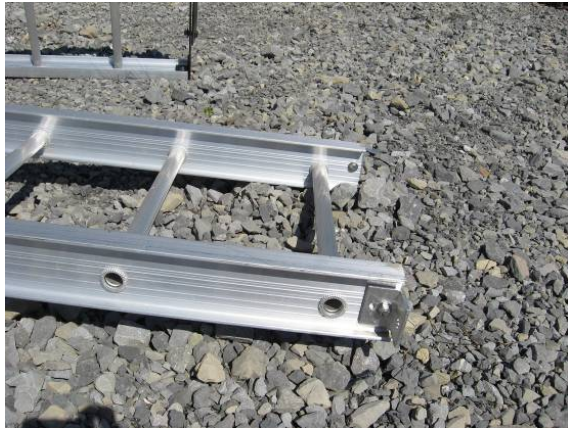
Anchor brackets located at the bottom of the ladder.
