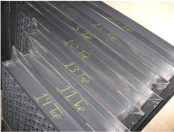
Louvers are numbered with the top identified. Each opening on the sump has a matching louver number.
