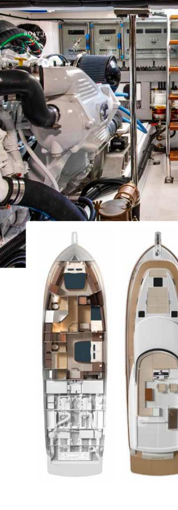
hatch on the aft deck. Each thru-hull fitting, hose and wire run is labeled. There is 4 feet, 8 inches of headroom and easy access around the Cummins diesels. Cleaning out the water strainers, checking the vacuum gauges on the dual fuel and water separators, and other routine maintenance should keep this space looking new when the boat is 10 years old.
