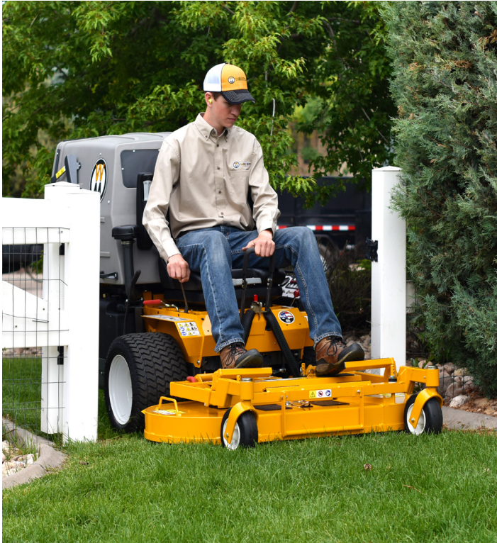
Walker T27i with 52" deck footprint: 53" (134.62 cm) W 95" (241.30 cm) L versus a Z Master with 52" deck: 68" (172.72 cm) W 102" (259.08 cm) L
