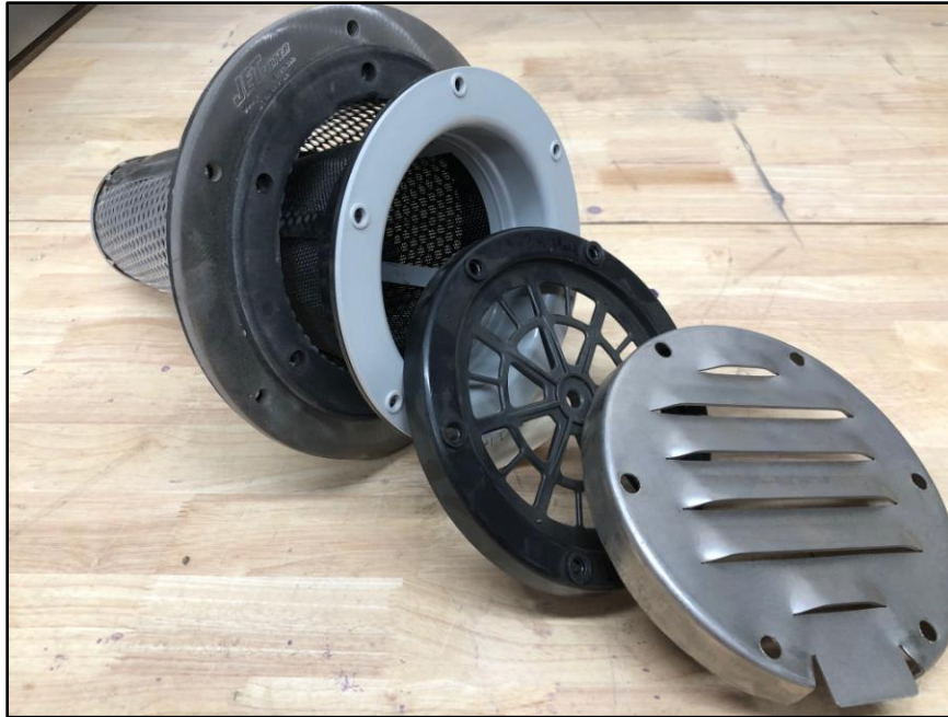
Figure 6. "Open-End" Component Assembly for Drainage Flow Testing Only
