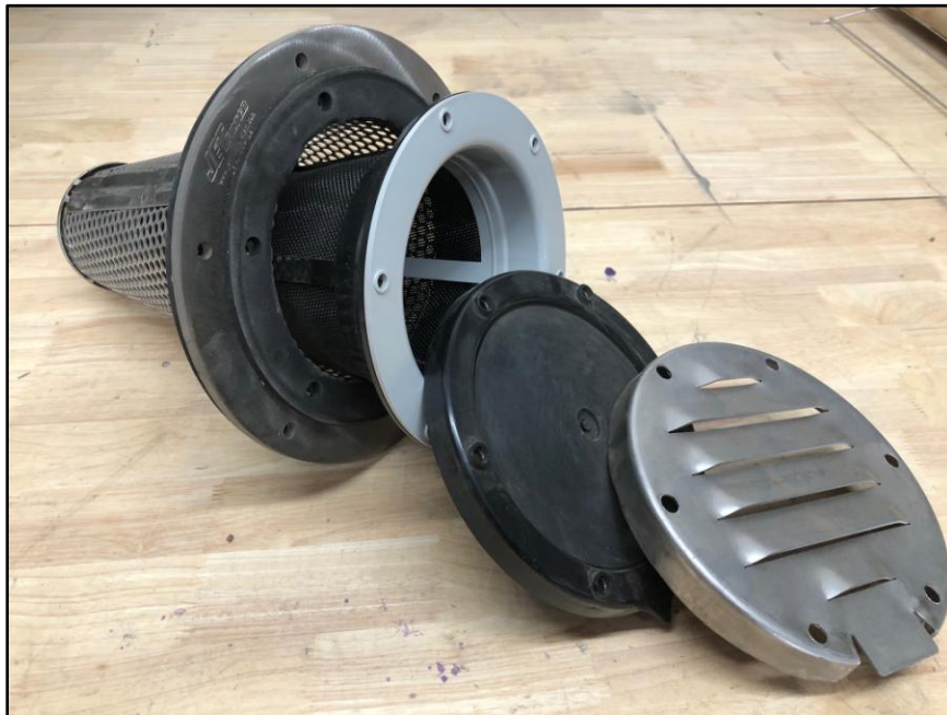
Figure 7. "Closed-End" Component Assembly for Reverse Flow Testing includes a Back-flow Prevention Valve
