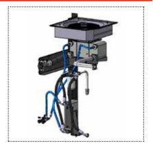
RVX 55-90i W compressors are equipped with water-cooled plate style heat exchangers. One is an oil cooler and the other an aftercooler. A dedicated cooling fan provides heat exchange for the cabinet.
