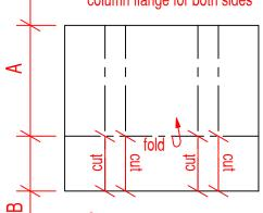
Step 2. Cut, Fold & Apply finger flashings at column web for both sides
